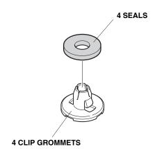
14. Install the four clip grommets into the four holes in the hatch. Press each grommet until you hear a click.
