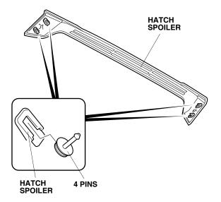
16. Using a utility knife, cut two slits in the adhesive backings on the hatch spoiler.
